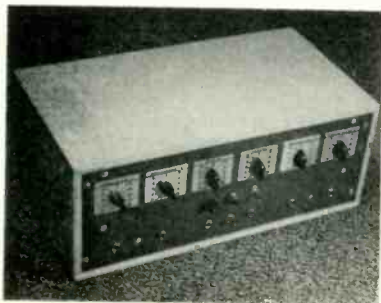
Fig. 1. Six-position stereo mixer that doubles as a portable unit.
